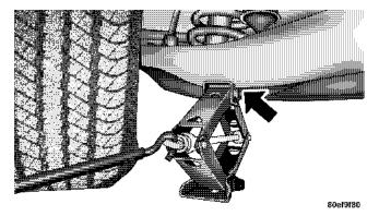
• Operate the jack using the jack drive tube and the wheel wrench. The tube extension, may be used, but is not required.
